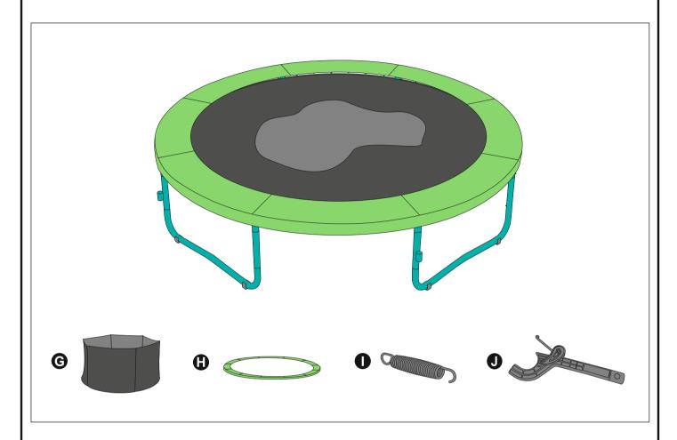
The Trampoline Mat (G) has metal rings with red markings, which should be the first ones using springs to connect to the frame of the upper structure. These rings with red markings should be on each side of the Vertical Leg A and match up with the posted upward-arrow red stickers.
