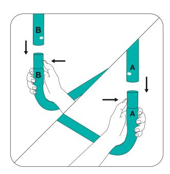
(4) Insert the base structure completed in Step 3 into the T-Connector (E) from Step 1. Ensure that the spring-loading pins of the vertical legs are inserted into the T-connectors correctly.
