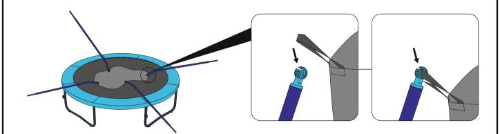
(12) Insert the Lower Frame Support with Foam (L) into the outward-facing metal cube on the Vertical leg A as shown in 12.1. After that, follow the provided sequence to secure the frames and legs using the Screw Set (M). The Screw Set is composed of four parts, each of which will be used in different positions as shown in 12.2 to 12.9.
