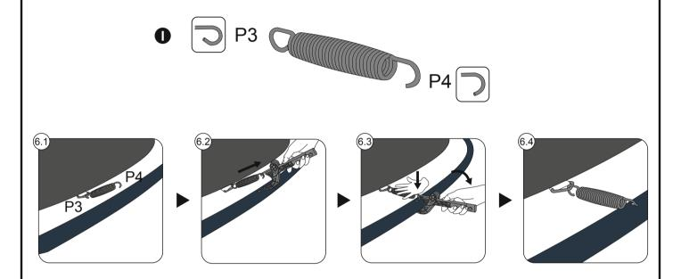
(7) Connect the metal rings to the frame on each side of Vertical Legs B.
