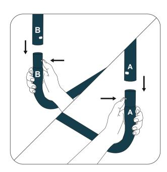
(4) Insert the base structure completed in Step 3 into the T-Connector (E) from Step 1. Ensure that the spring-loading pins of the vertical legs are inserted into the T-connectors correctly.
