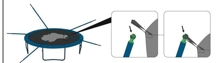
(12) Insert the Lower Frame Support with Foam (L) into the outward-facing metal cube on the Vertical leg A as shown in 12.1. After that, follow the provided sequence to secure the frames and legs using the Screw Set (M). The Screw Set is composed of four parts, each of which will be used in different positions as shown in 12.2 to 12.9.
