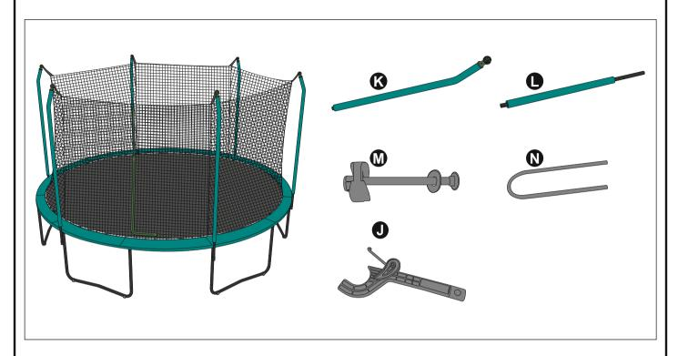
10 Insert the Lower Frame Support with Foam (L) into the Upper Frame Support with Support Cap (K).
