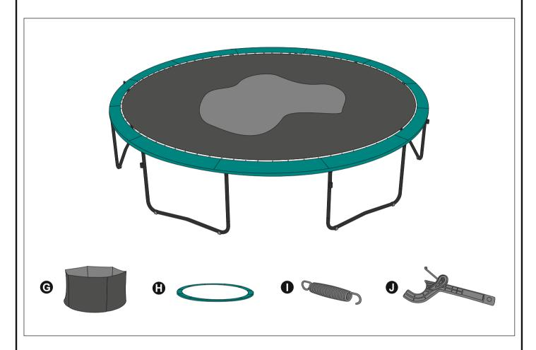
(5) The Trampoline Mat (G) has metal rings with red markings, which should be the first ones using springs to connect to the frame of the upper structure. These rings with red markings should be on each side of the Vertical Leg A and match up with the posted upward-arrow red stickers.
