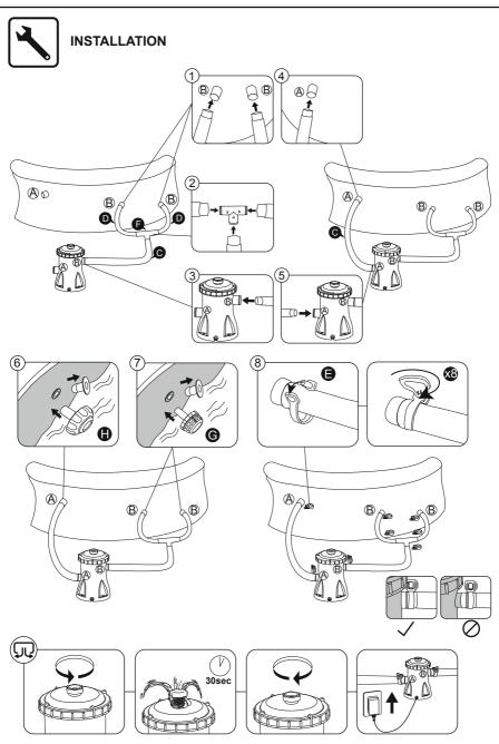
**AIR DISCHARGING OPERATION:** Follow these steps to discharge air before switching the filter pump on and after every maintenance operation. Omitting this operation will greatly affect the lifespan of the product.
