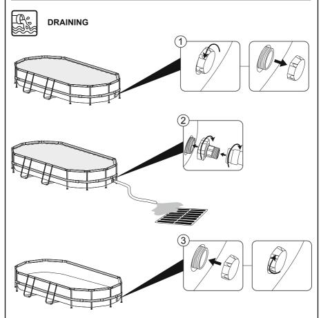
For draining, follow the illustrations. Drawings are for illustration purposes only. May not reflect actual product. Not to scale. Before draining your pool water, make sure that you are draining your pool away from the house and any objects that are subject to water damage. Check local regulations for drainage by laws.
