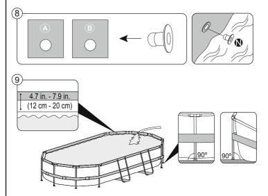
**IMPORTANT:** Check the position of the vertical legs at times while filling the pool with water. The legs can gradually change position due to increased water weight. If the legs are not perpendicular to the ground, please stop filling the pool and adjust them. It will help with weight distribution to avoid strain on the frame and liner.
