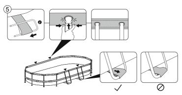
Fully extend the support sleeves on the bottom of the liner to ensure the correct positioning of the U supports.
